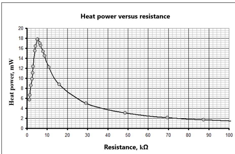
To determine the position of the maximum, it is necessary to take additional measurements in the range of 0 to 10 kΩ. According to the measurement results, it turns out that the maximum heat power generated in the resistor is reached at
