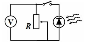
**1.2 – 1.5** The results of the measurement of the voltage across the resistor as a function of its resistance are shown in Table 1. It also presents the results of calculations of the current using the formula
