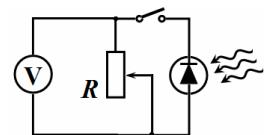
**1.2 – 1.5** The results of the measurement of the voltage across the resistor as a function of its resistance are shown in Table 1. It also presents the results of calculations of the current using the formula
