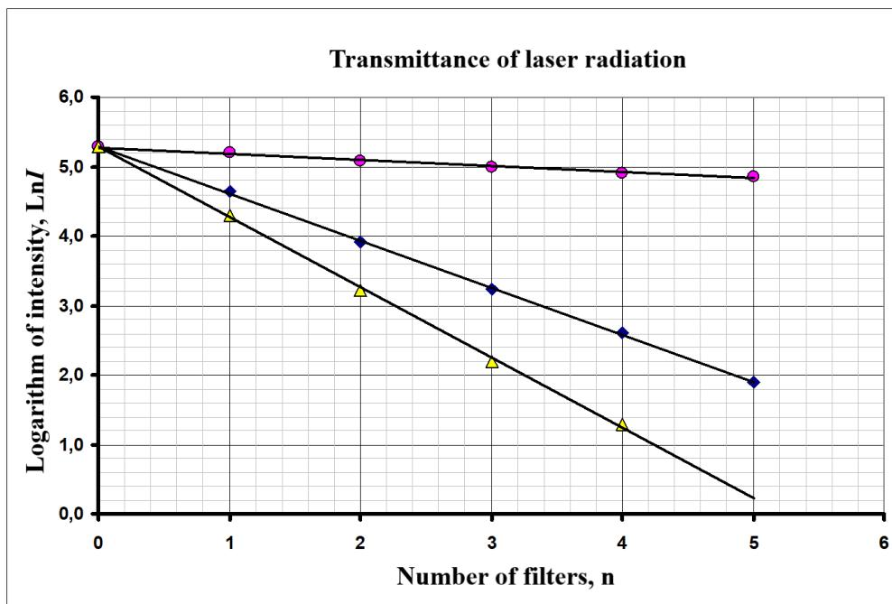
**2.3** As it follows from formula (5), the slope of the dependence is equal to the logarithm of the transmittance  $a = \ln k ,$  (6)
