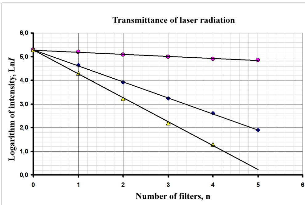
2.3 As it follows from formula (5), the slope of the dependence is equal to the logarithm of the transmittance
