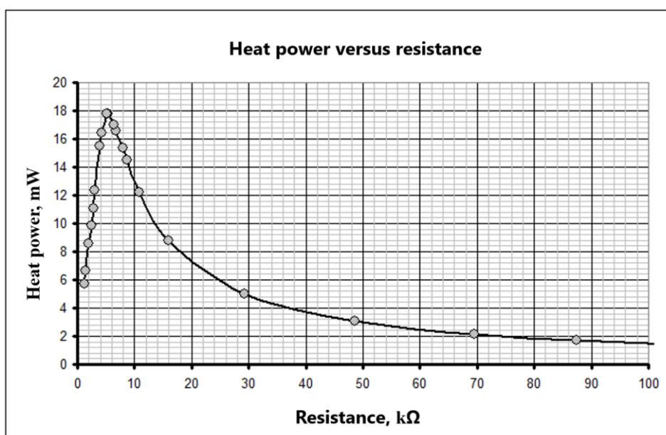
To determine the position of the maximum, it is necessary to take additional measurements in the range of 0 to 10 kΩ. According to the measurement results, it turns out that the maximum heat power generated in the resistor is reached at
